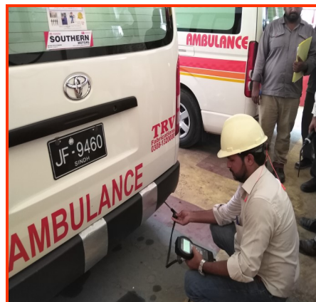
Vehicle Emission Monitoring
