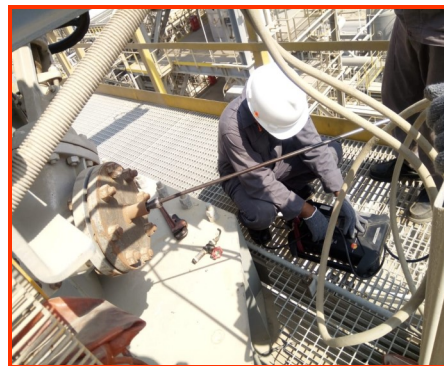
Stack Emission Testing
